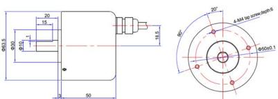
4. Connector /Dust and splash proofed with rear cable (CW type)
